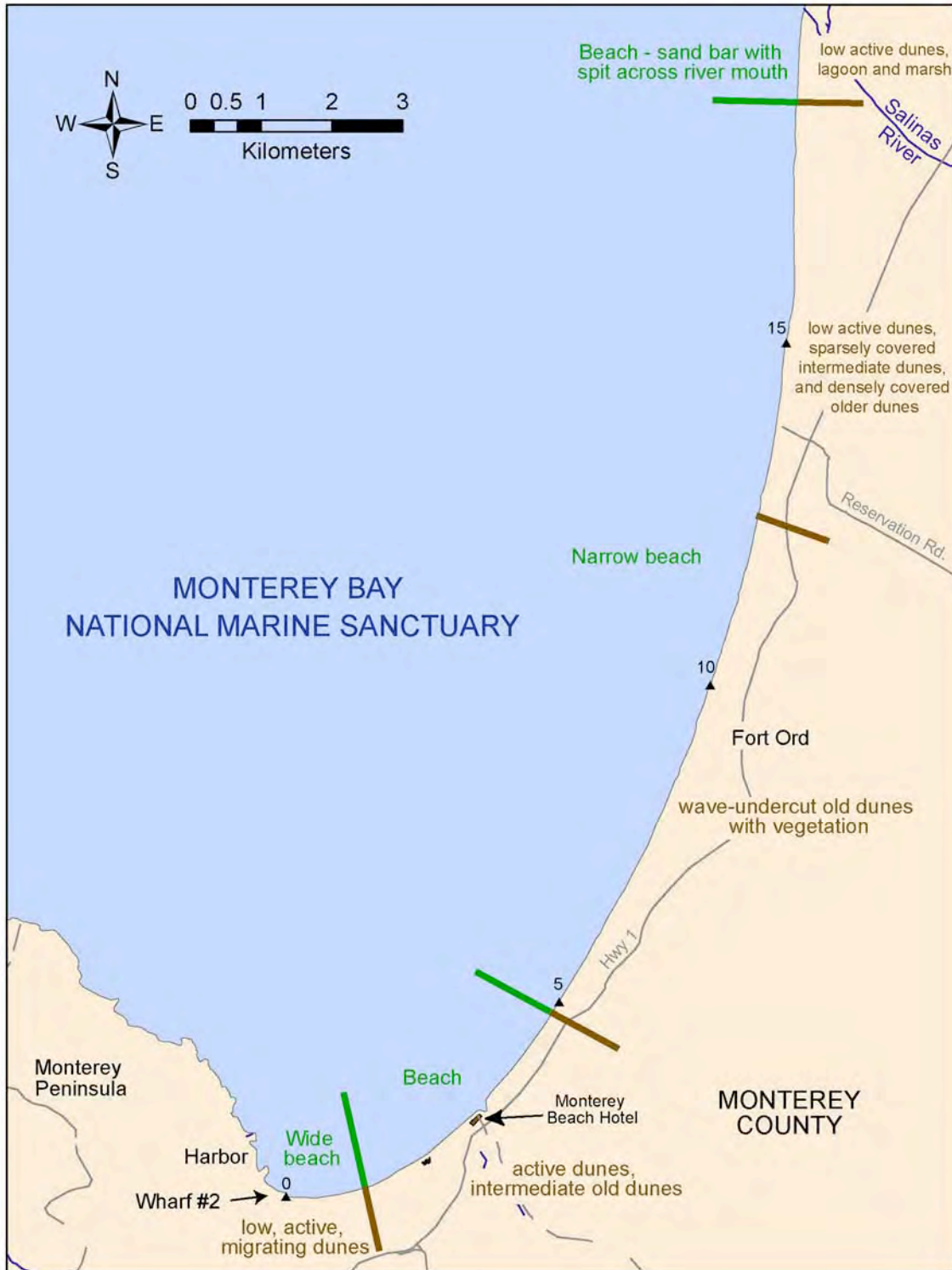
Figure 1.4: Relative beach width (green text) and adjacent dune morphology (brown text) in southern Monterey Bay. Distances from Wharf #2 in Monterey are shown in kilometers (black triangles). Coastline descriptions from Coyne (2001).
