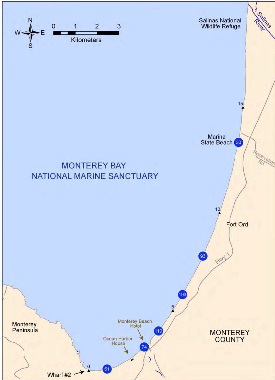
Figure 2.3: Coastal erosion rates in centimeters per year (blue circles) for the time period 1940-1984, as documented by Thornton et al. (in press). Distances from Wharf #2 in Monterey are in kilometers (black triangles). For reference, 100 cm=3.28 ft.
