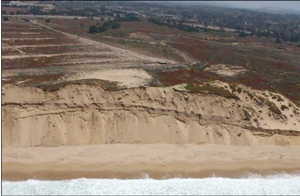
Figure 1.5: Aerial photograph of wave-cut dunes near the relatively undeveloped area of Fort Ord, California. This type of erosion provides much of the sand for the southern Monterey Bay littoral system. Despite the fact that this photograph was taken in summer, the beach is relatively narrow. During storms and/or high tides, waves wash up the beach and undercut the dunes. See Figure 1.4 for location of Fort Ord. Photograph copyright © 2002 Kenneth & Gabrielle Adelman ( http://www.californiacoastline.org/ ).
