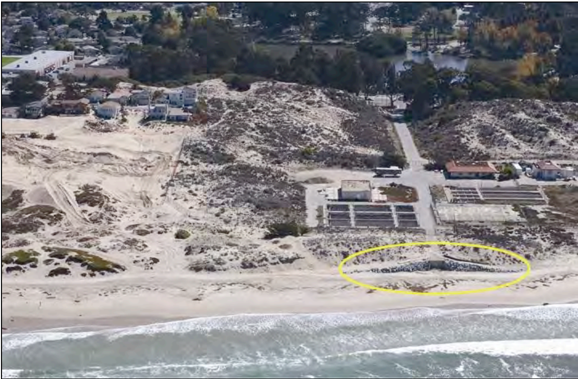
Figure 5.8: Aerial photograph of riprap on either side of a storm drain for the Naval Postgraduate School in Monterey, California. Photograph taken October 2004; copyright © 2002 Kenneth & Gabrielle Adelman ( http://www.californiacoastline.org/ ).
