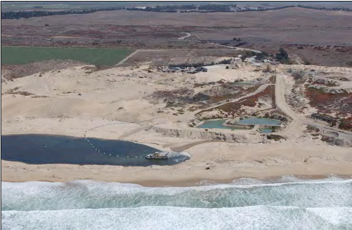
Figure 1.8: Sand mining operations in northern Marina, California. The company has dredged a lagoon from which they extract sand. Some argue that the lagoon actually traps beach material in addition to dune sand. See Figure 1.9 for location of mine. Aerial photograph taken in October 2004; copyright © 2002 Kenneth & Gabrielle Adelman ( http://www.californiacoastline.org/ ).
