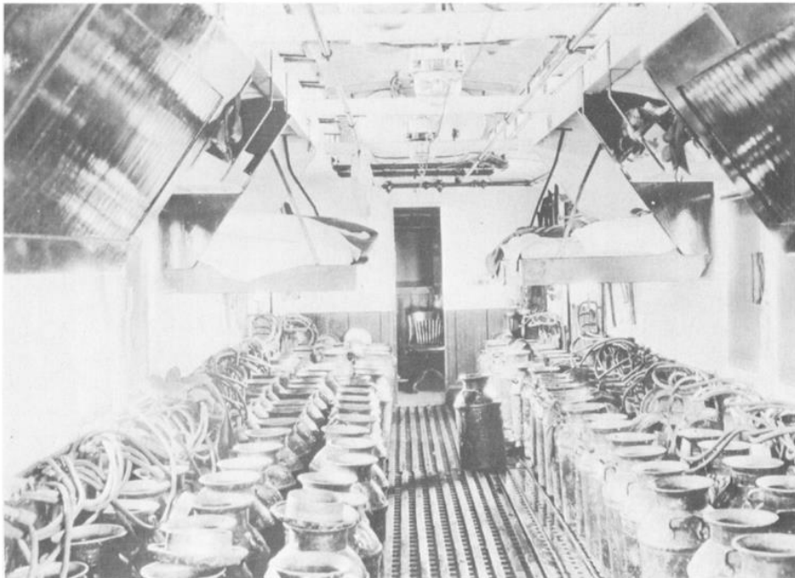
FIGURE 29. Interior of railroad fish distribution car. Hoses supplied air to the cans containing fish. Bunk beds provided sleeping accommodations for crew members.
