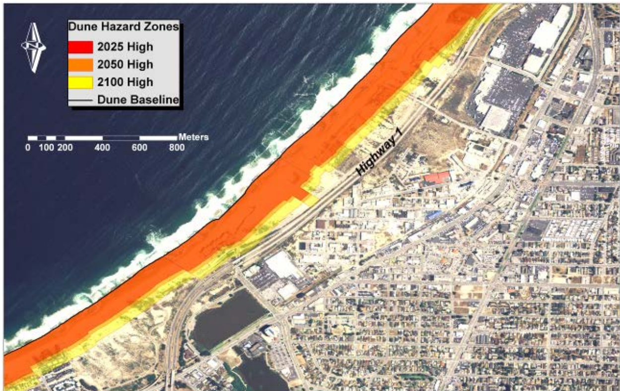
Figure 23 Erosion Hazard Zones similar to those used to delimit development setbacks
