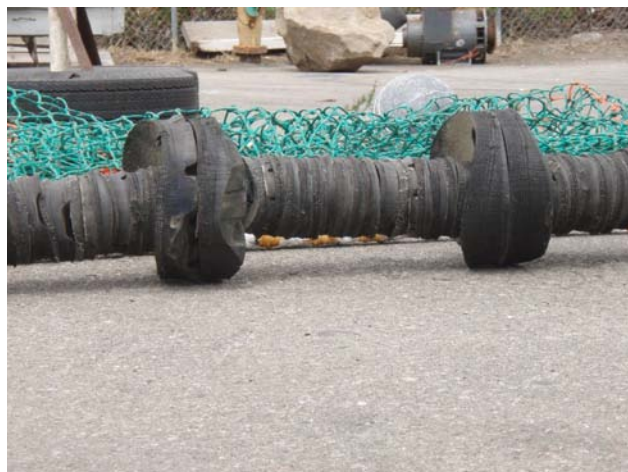
Figure 3. Picture showing the groundgear with both 8 in. and 4 in. discs.
