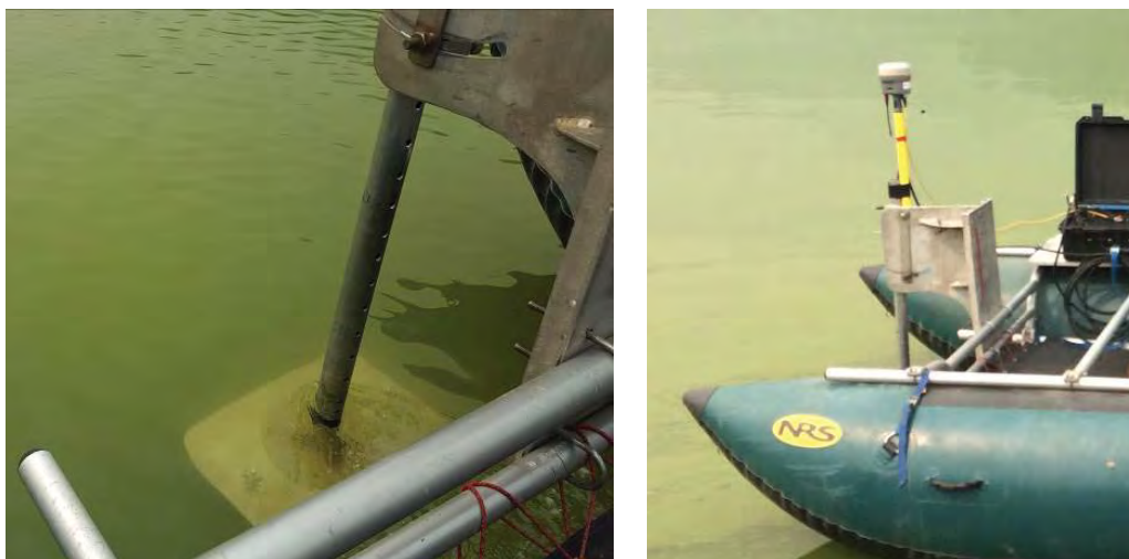
Figure 5. SBE (below water) with collocated RTK GPS (top of pole).
