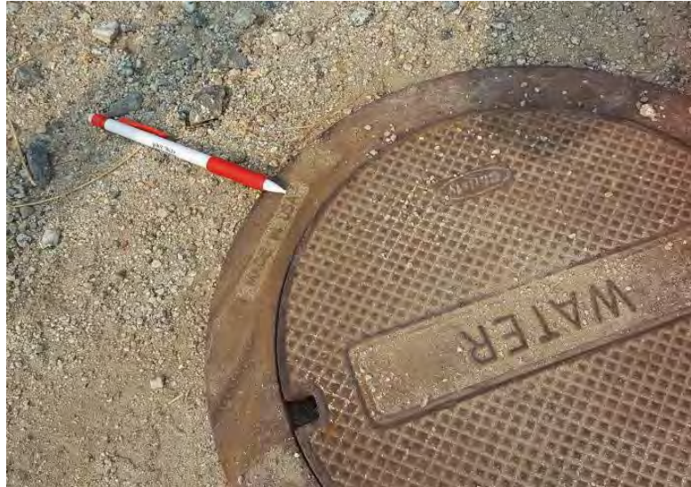
Figure 2. HDR benchmark is the top of the Letter “A” located at the end of the pencil in this figure.
