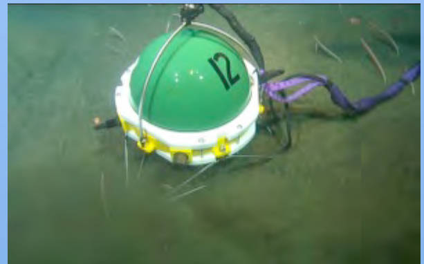
Seismometer housing deployed off launch frame
