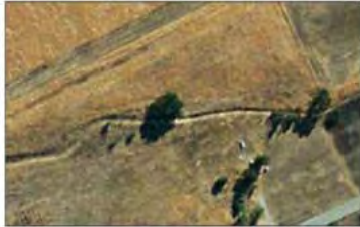
Figure 4.4. Example of a stream reach with a low vegetation density that does not provide SRA or root mass capable of withstanding erosion during high flow events.
