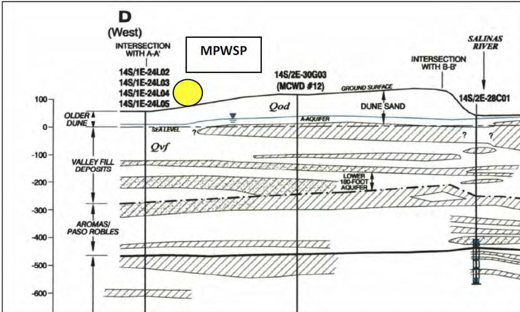
Figure 13. Geologic Cross-Section (Portion of Plate 6 from HLA, 2001)
