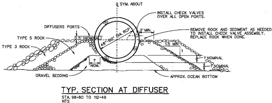
**Figure C1. Typical diffuser section (currently in place).**
