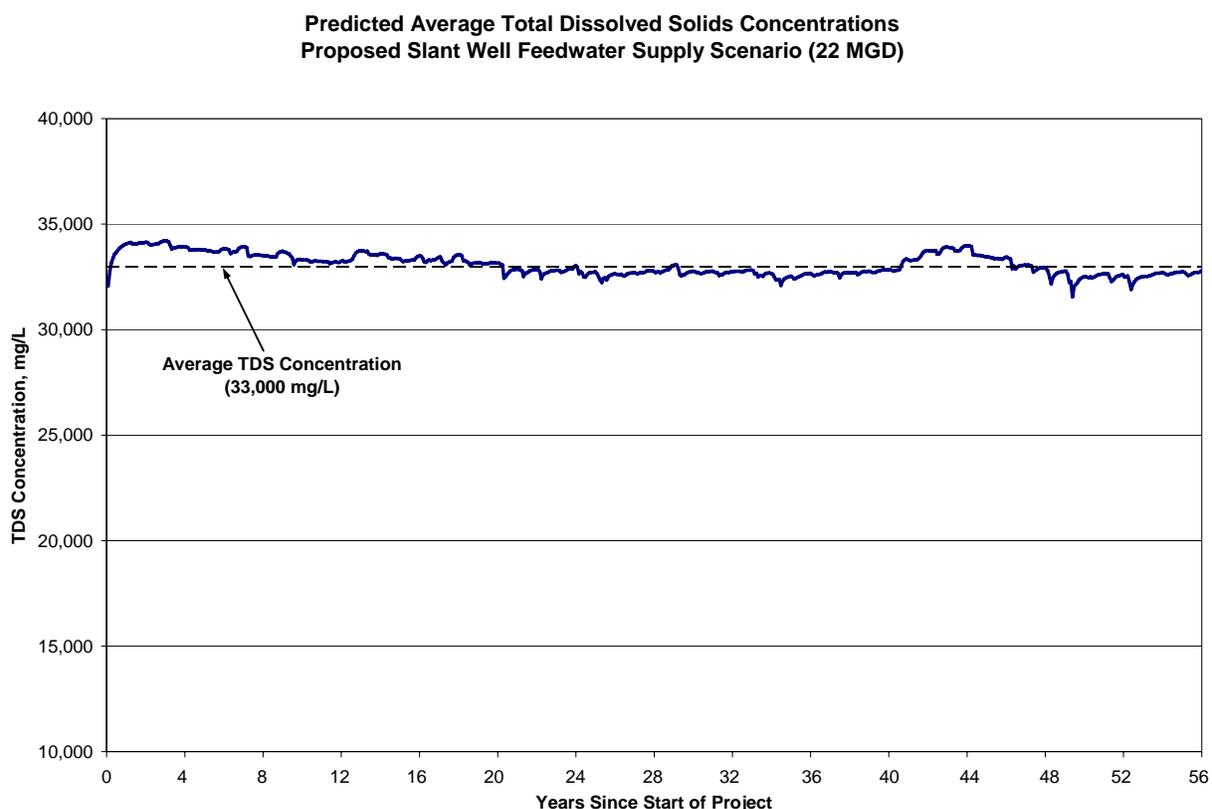
The predicted TDS concentration of 33,000 mg/L for the feedwater extracted by the six slant wells is approximately 94 to 97 percent of the TDS concentration of seawater (34,000 to 35,000 mg/l). As the modeled layout represents a worse-case scenario (due to the steeper well angles), the most recent layout (six 700 ft wells with a 20 degree angle proposed by RBF, 2008) would most likely result in an even higher percentage of seawater in the extracted water.
