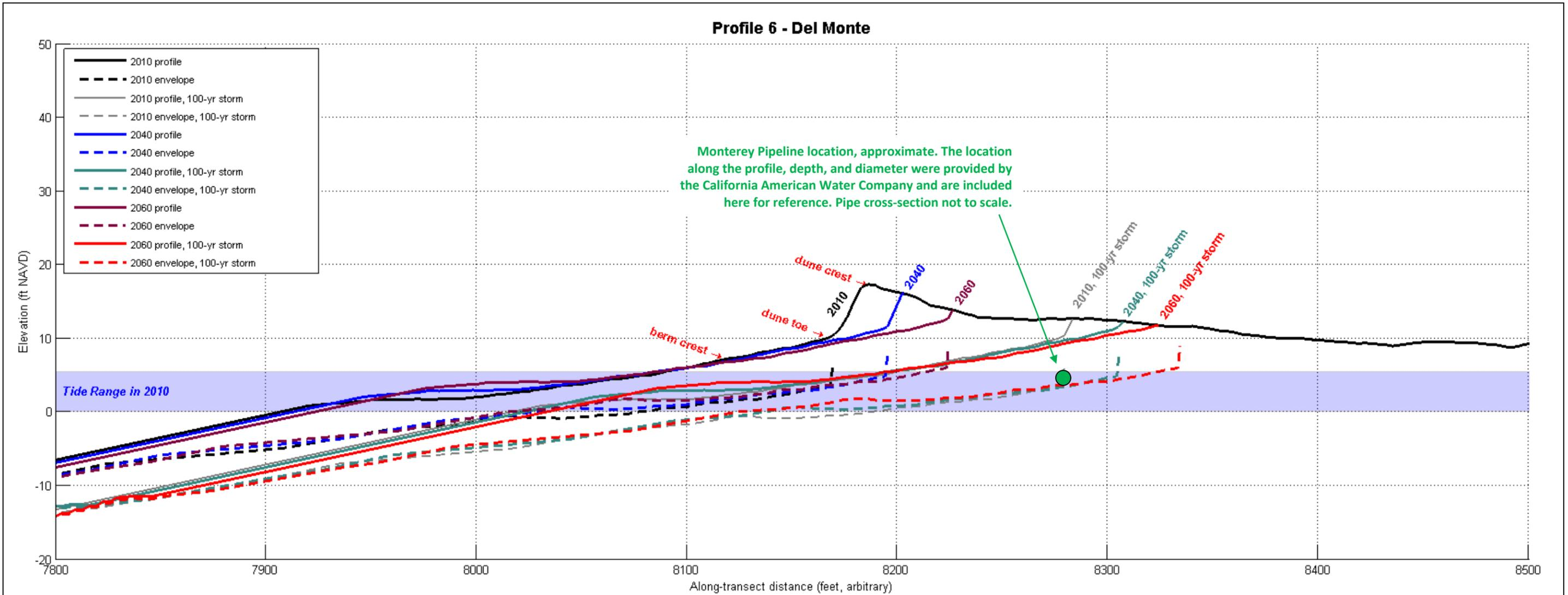
Monterey Pipeline location, approximate. The location along the profile, depth, and diameter were provided by the California American Water Company and are included here for reference. Pipe cross-section not to scale.
