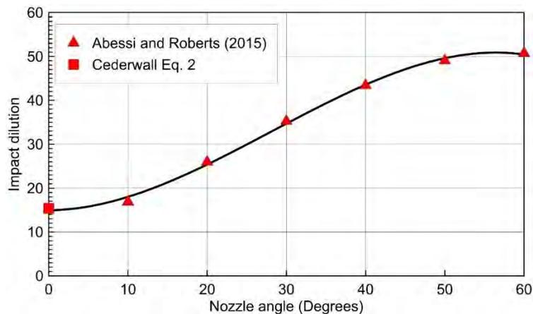
**Figure 7. Effect of nozzle angle on dilution of dense jets, case T2.**
