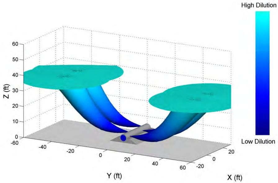
**Figure 8. An illustration of the positively buoyant effluent plumes of Analysis 3.1.
