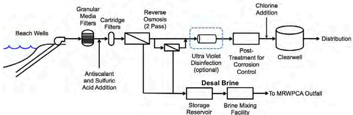
Figure 1 – Schematic of CalAm desalination facilities
