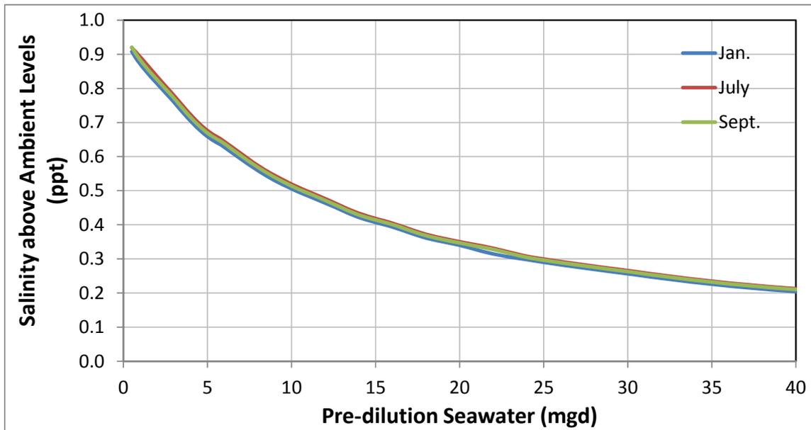
**Figure C9. Simulated seafloor salinity (ppt above ambient salinity) for desalination brine (13.84 mgd) as a function of the flow rate of pre-dilution seawater; results calculated using the Visual Plumes method.**
