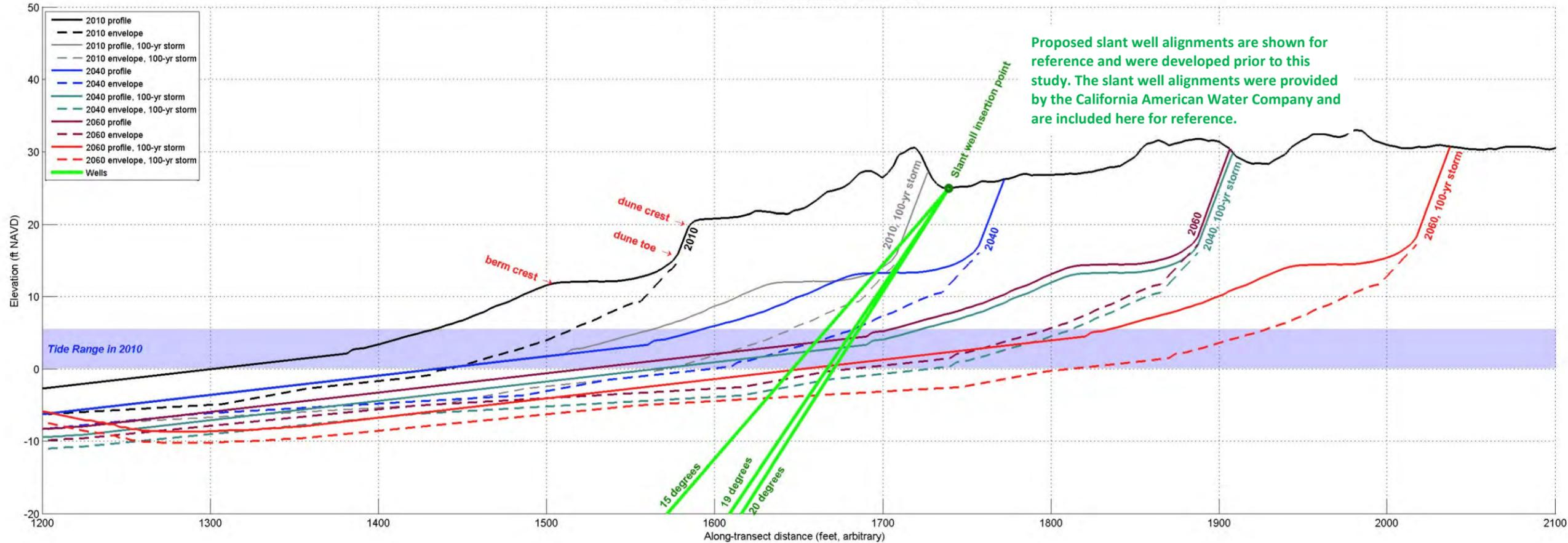
Proposed slant well alignments are shown for reference and were developed prior to this study. The slant well alignments were provided by the California American Water Company and are included here for reference.
