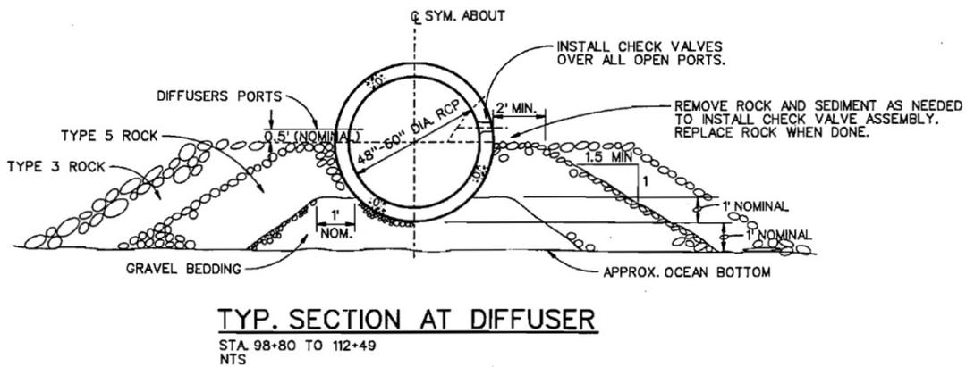
**Figure 1. Typical diffuser section (currently in place).**
