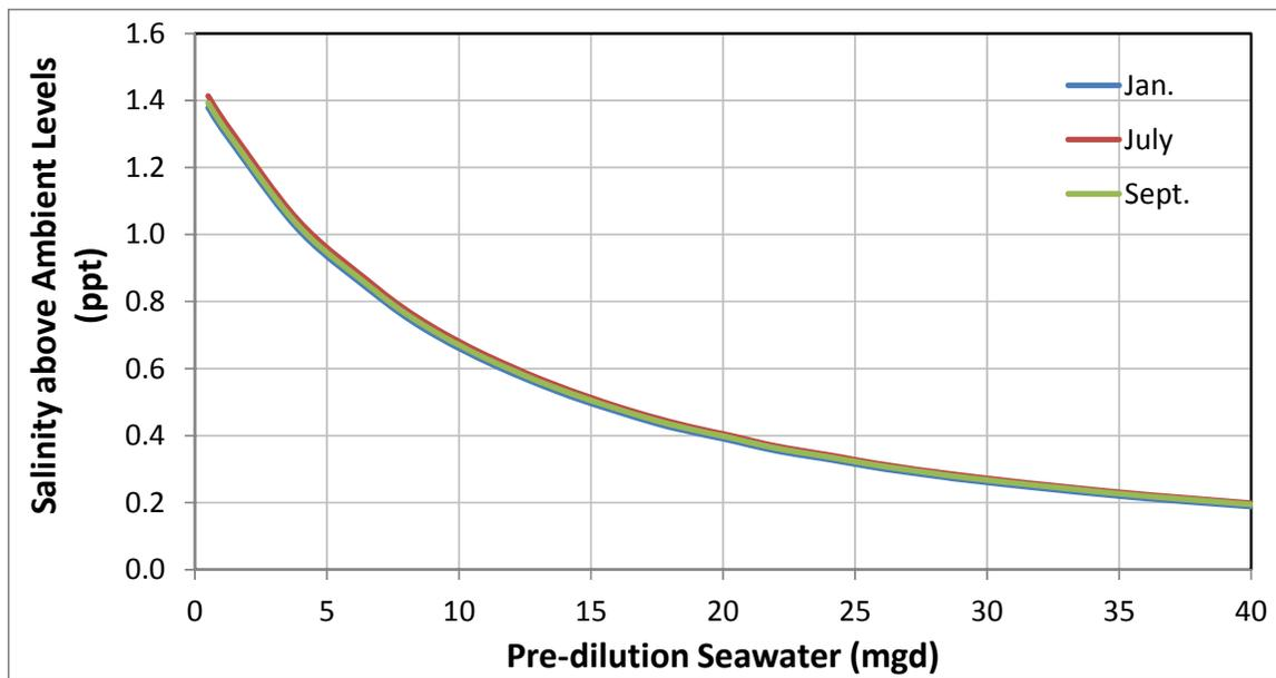
**Figure C8. Simulated seafloor salinity (ppt above ambient salinity) for desalination brine (13.98 mgd) as a function of the flow rate of pre-dilution seawater; results calculated using the semi-empirical method.**
