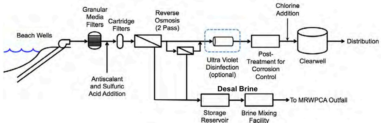
Figure 1 – Schematic of CalAm desalination facilities
