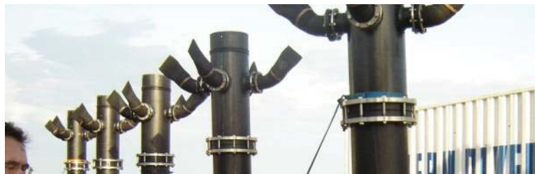
Figure 6-3. A rosette multiport brine diffuser.
