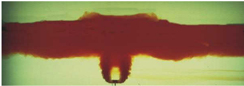
Figure 14. Trapped buoyant plume from multiport diffuser in stratified environment, from Roberts et al. (1989).
