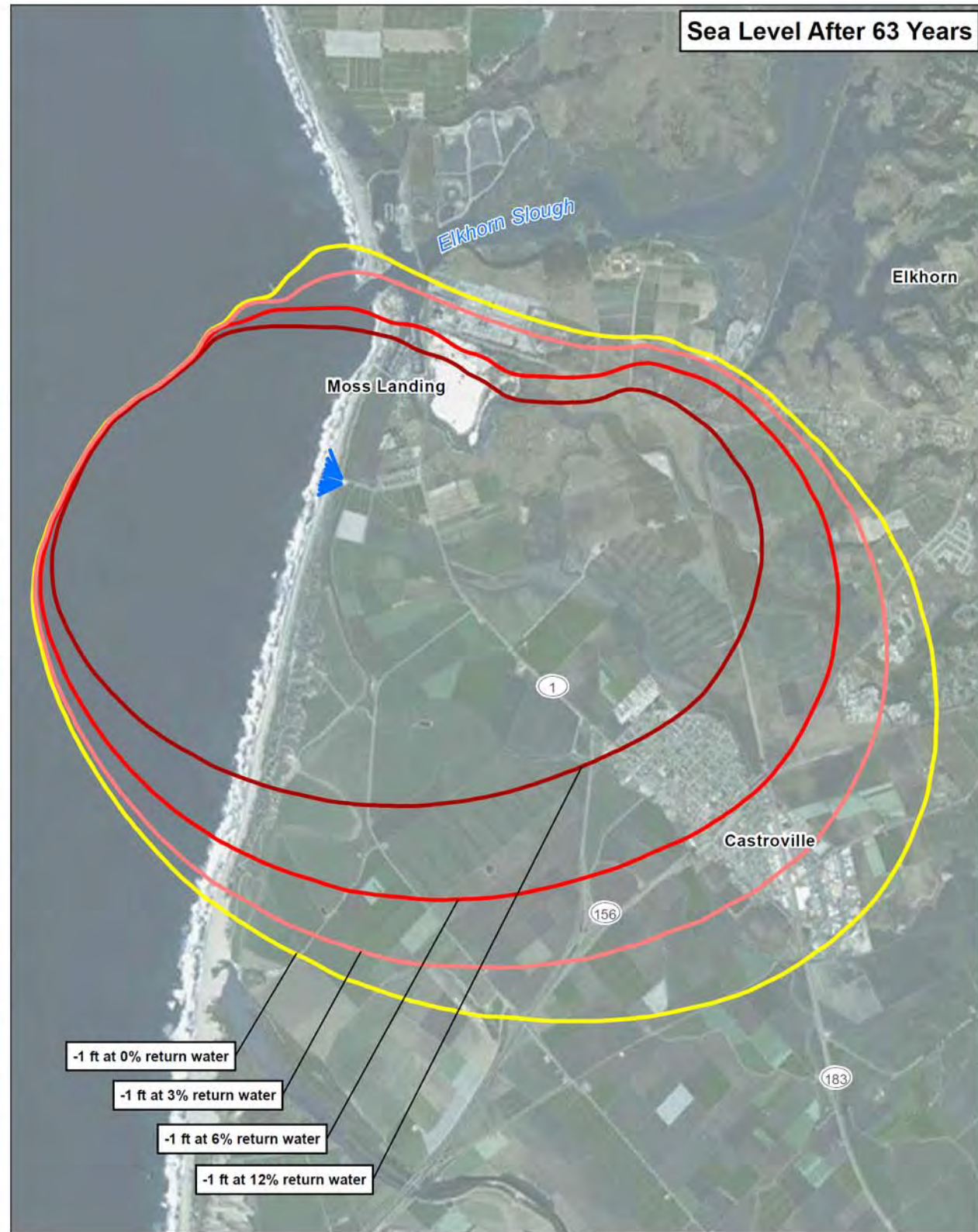
205335.01 Monterey Peninsula Water Supply Project Figure 5.5-3 Potrero Rd Slant Wells: 1-Foot Response in 180-Foot Aquifer under 24.1 MGD Pumping
