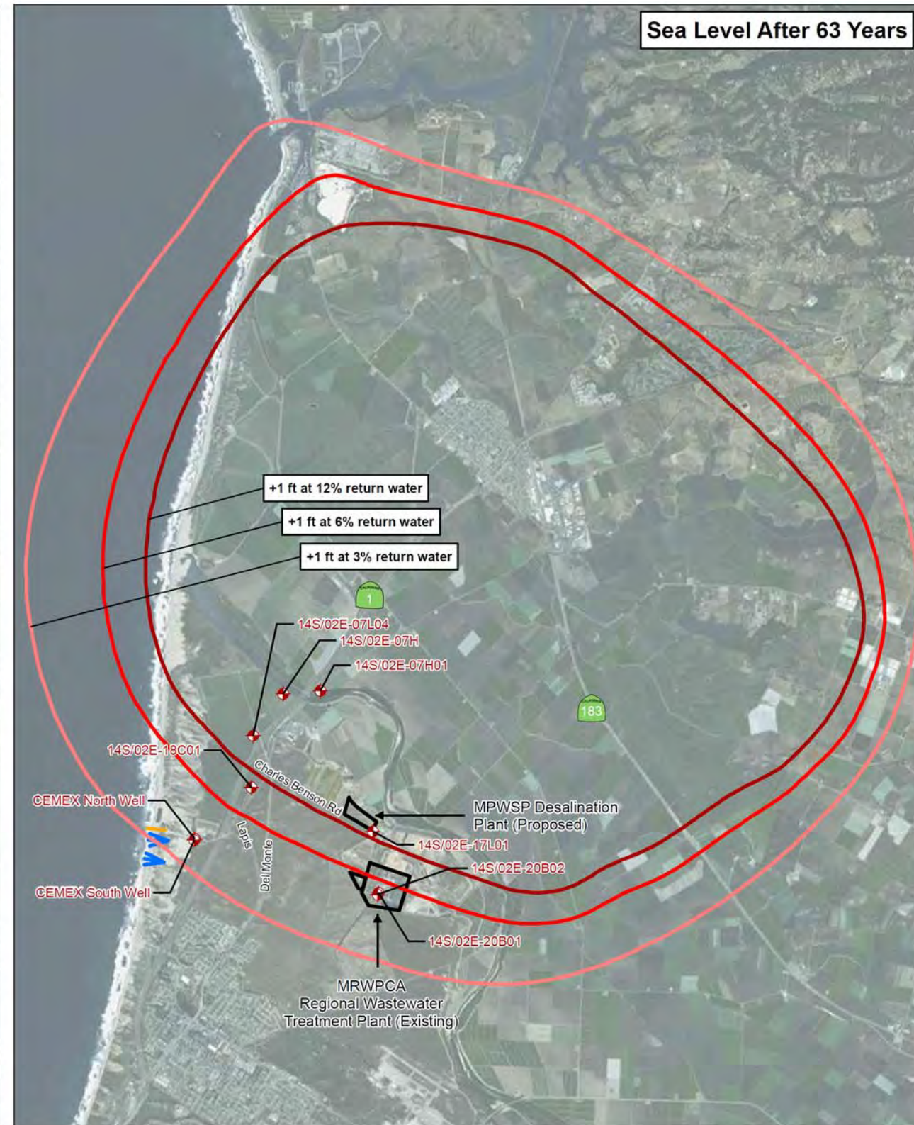
205335.01 Monterey Peninsula Water Supply Project Figure 5.5-7 Alternative 5a Site: 1-Foot Response in 400-Foot Aquifer under 15.5 MGD Pumping
