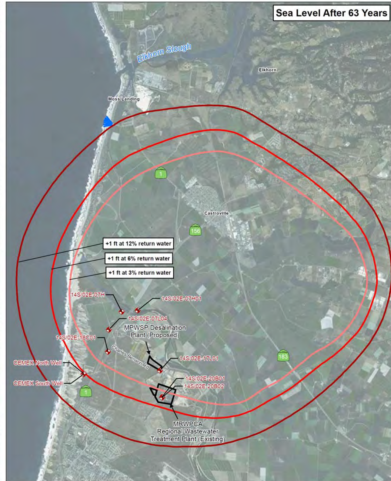
205335.01 Monterey Peninsula Water Supply Project Figure 5.5-10 Alternative 5b Slant Wells: 1-Foot Response in 400-Foot Aquifer under 15.5 MGD Pumping
