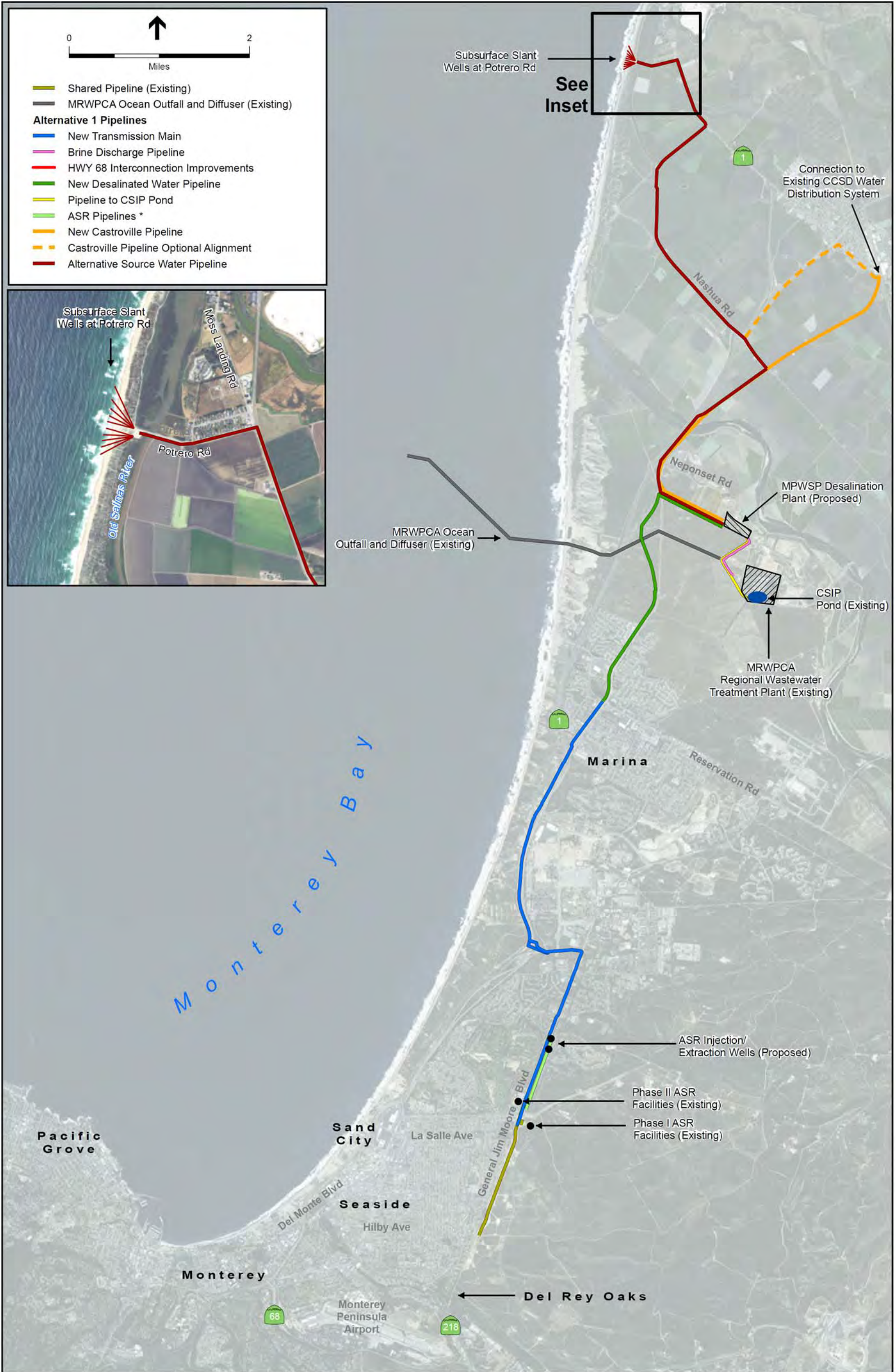
205335.01 Monterey Peninsula Water Supply Project Figure 5.4-1 Alternative 1- Slant Wells at Potrero Road
