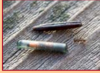
11.5 mm long PIT tag with grain of rice
