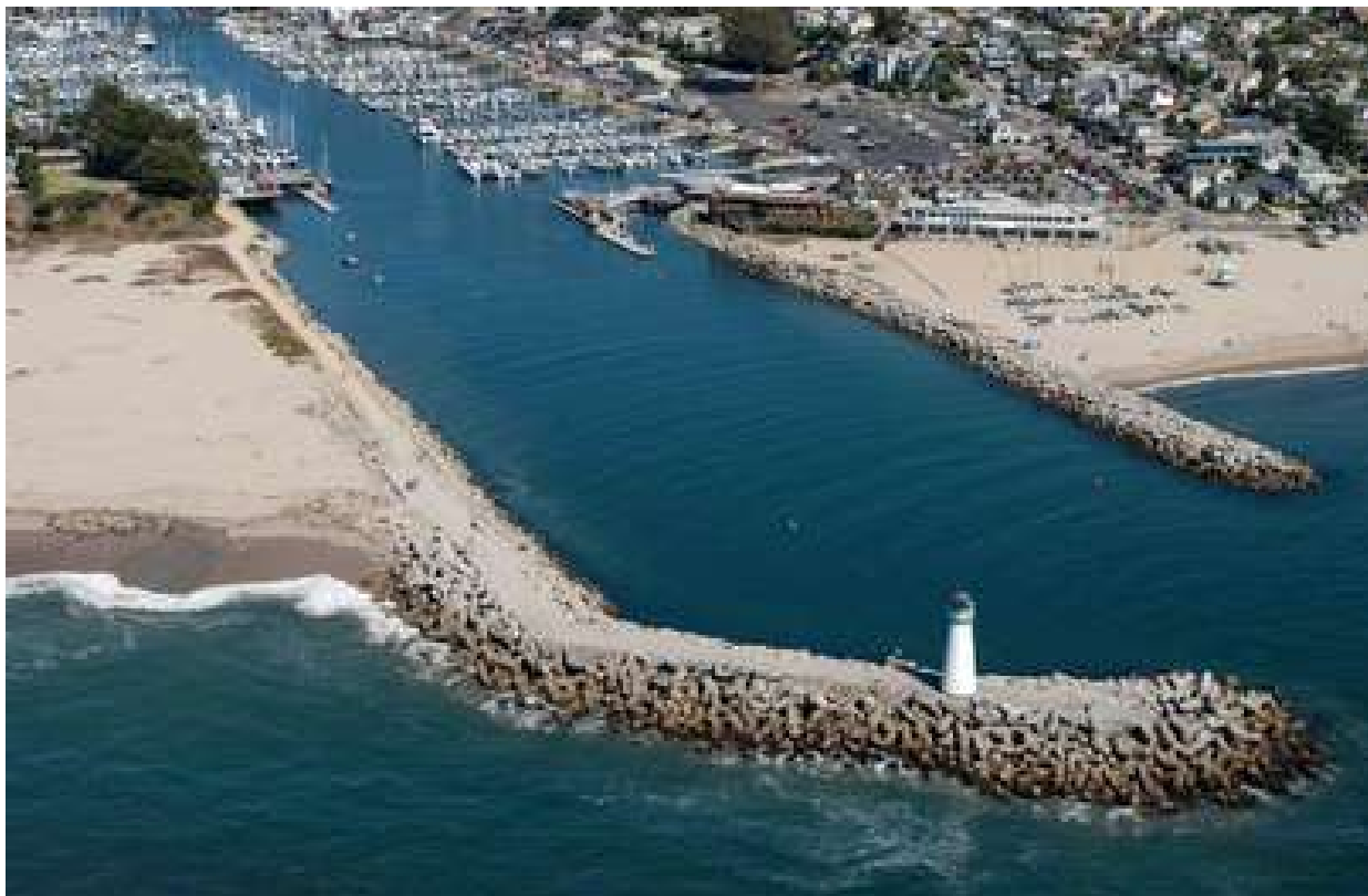
Figure 4-7. Aerial view of the two jetties that stabilize the entrance to Santa Cruz Harbor. Source Adelman and Adelman (2013)
