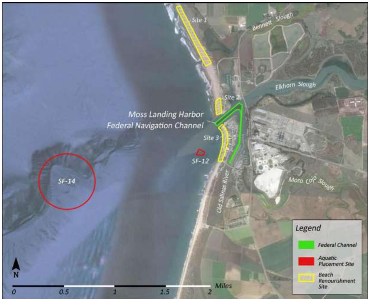
Figure 2-13. Moss Landing dredged material placement sites and beach nourishment sites. Source: USACE, 2014c
