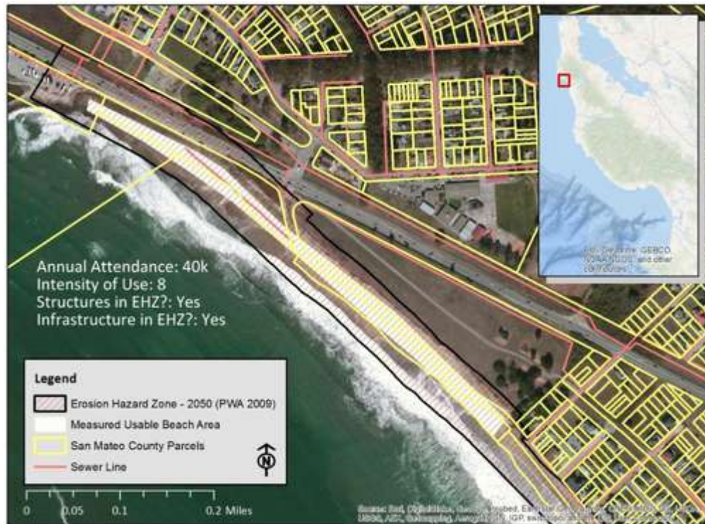
Figure 7-1. Erosion hazard zone - Surfer's Beach area
