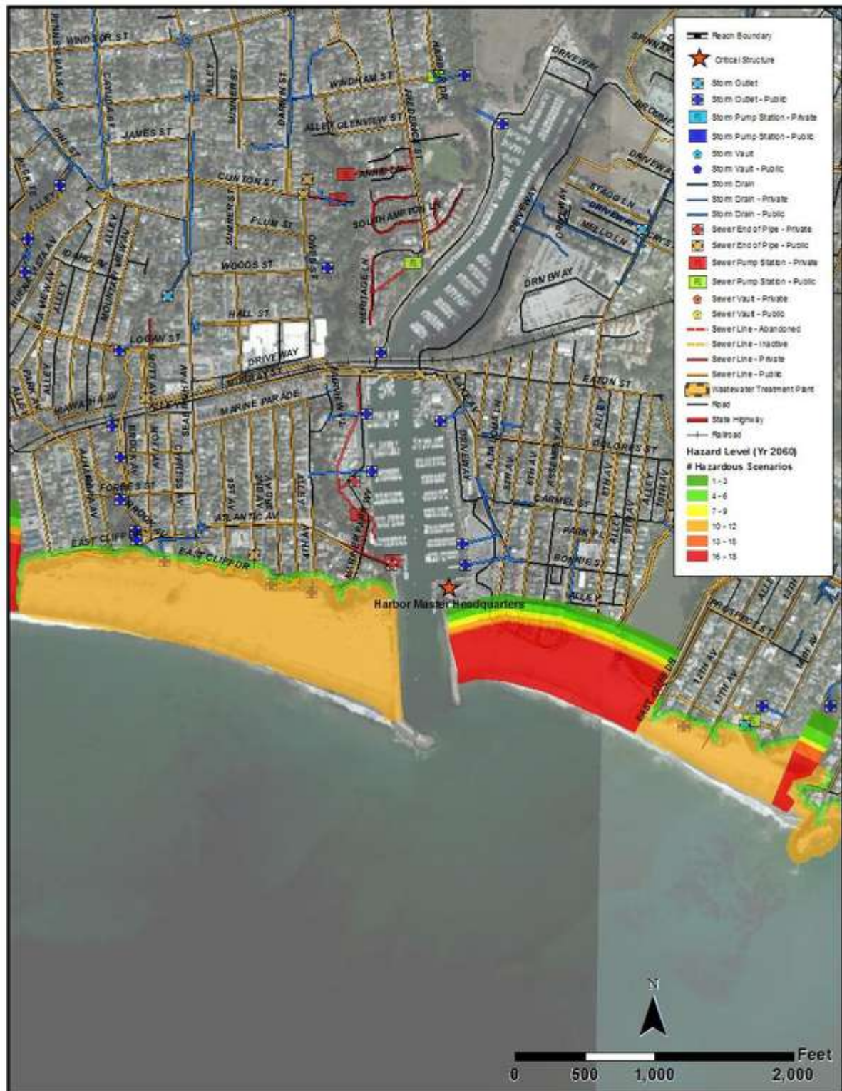
Figure 3-2. Scenario based coastal erosion hazard zones (ESA-PWA, 2014) and vulnerable infrastructure (City of Santa Cruz, County of Santa Cruz) at Santa Cruz Harbor and Twin Lakes State Beach. The scenario based hazard zones are a spatial aggregation of dune erosion, cliff erosion, tidal inundation, and storm flood hazard zones.
