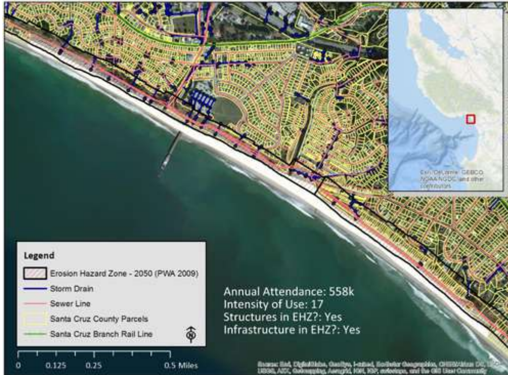
Figure 7-15. Erosion hazard zone - Seacliff State Beach
