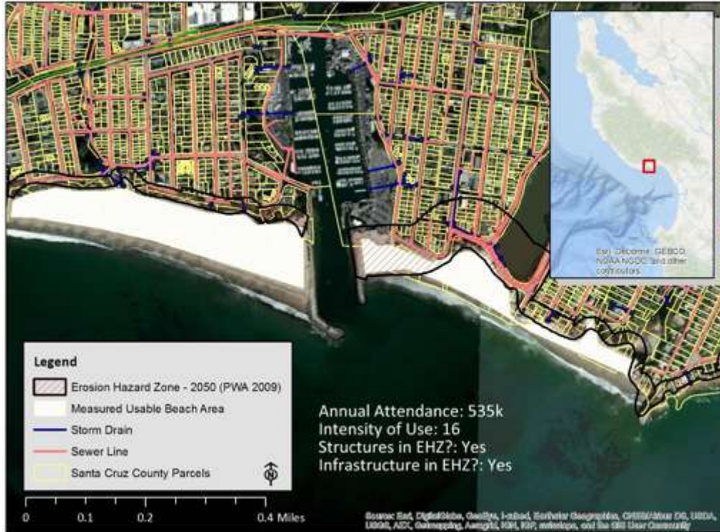
Figure 7-10. Erosion hazard zone - Twin Lakes State Beach
