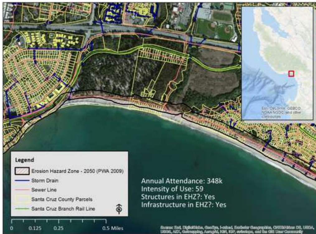
Figure 7-14. Erosion hazard zone - New Brighton State Beach
